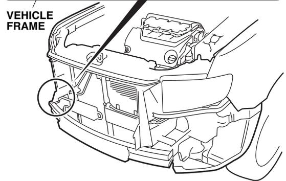
9. Secure the fog light harness ground terminal to the vehicle frame with one ground bolt.
