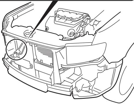
7. Plug the fog light harness 1-pin connector into the vehicle 1-pin connector.
