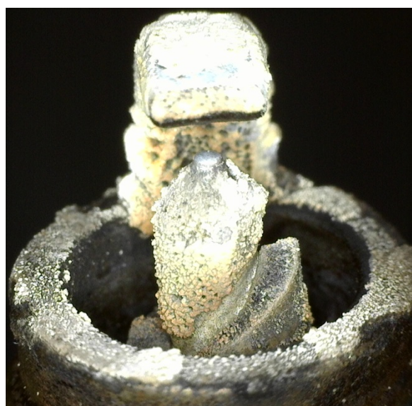
No good: Insulator badly broken
